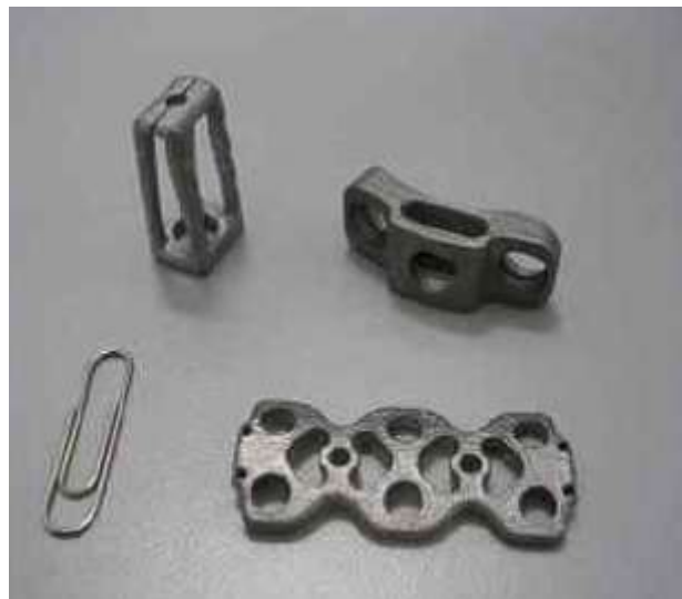
Figure 20. Examples of parts built in EOS Titanium Ti64 for vertebral column prostheses
