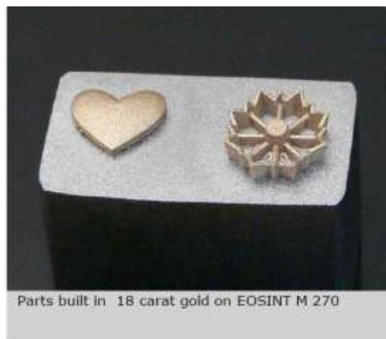
Figure 9. Example of new materials used (gold)
