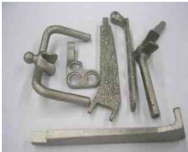
Figure 19. Examples of parts built in EOS Titanium Ti64
