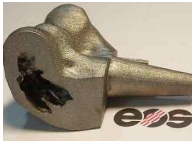
Figure 21. Examples of parts built in EOS Titanium Ti64 for orthopededy implants
