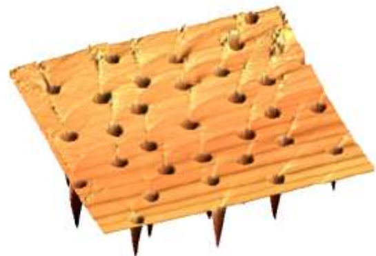
Figure 2: Typical geometrical defects of cleaved hollow fiber or capillary – left [www.crystal-fibre.com], AFM scan of cleaved hollow fiber visualizing surface geometrical defects– right [16]
