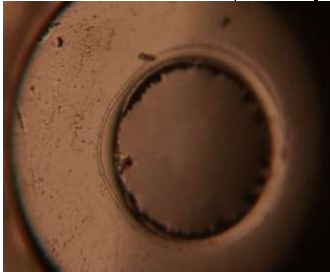
Figure 1: Capillary tip meniscus shape affected by capillary inner edge defects and impurities
