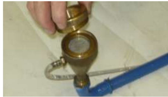
Figure 6. Case fixed inside the FBG.
