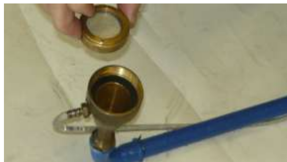
Figure 4. The case containing the disk is introduced in the FBG.
