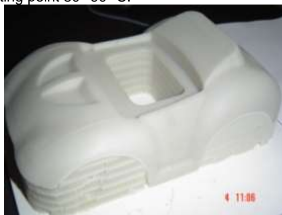
Figure 6. Body outline of a car built by thermojet technique.
