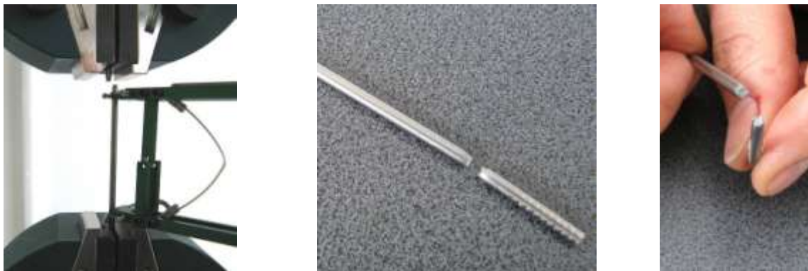
Figure 11 – Fracture of titanium uncoated specimen
