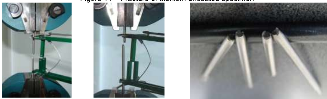
Figure 12 – Fracture of titanium carbon coated specimen a) Specimen 1 of titanium carbon coated; b) Specimen 2 of titanium carbon coated; c) Fracture zones of specimen 1 and 2
