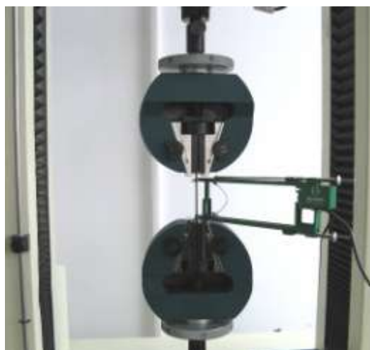
Figure 7 – Specimen in tensile test
