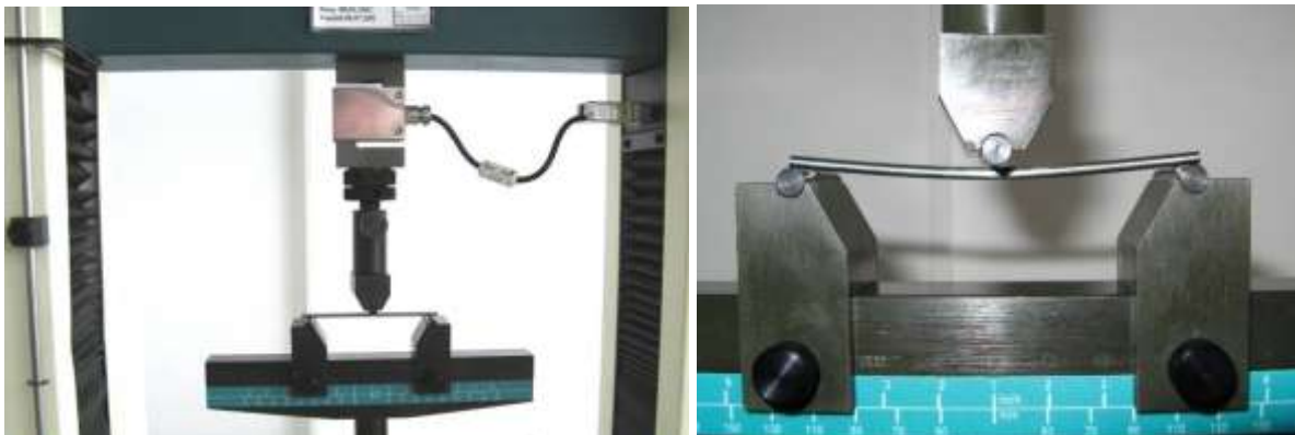
Figure 3 – Samples during bending test
