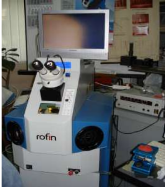
Fig. 3: The laser equipment used for remelting and the image of the remelting process
