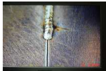
Figure 9. Examples of welded parts in CNC mode using ROFIN SW6002 laser installation.
