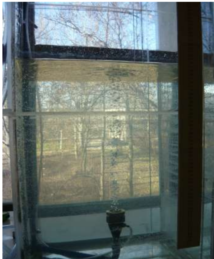
Fig. 7. Fine bubbles generator introduced in a water basin ( h = 0.5 m)
