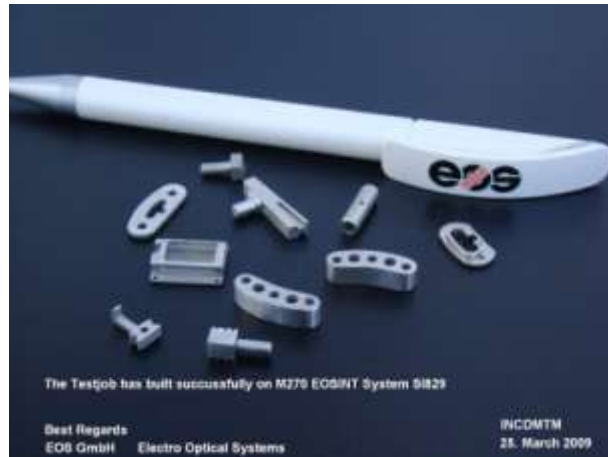
Figure 17. Examples of parts built in EOS superalloy CoCr MP1 on INCDMTM for orthopedy, neurosurgery and maxillofacial implants
