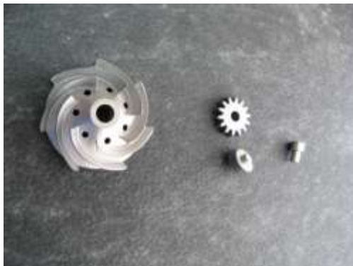
Figure 16. Examples of parts built in EOS superalloy CoCr MP1 on INCDMTM for industry
